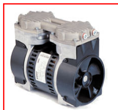
Twin cylinder piston vacuum pump or compressor 250 W motor developing 2.8 bar with flow to 8.7 m 3 /hr
