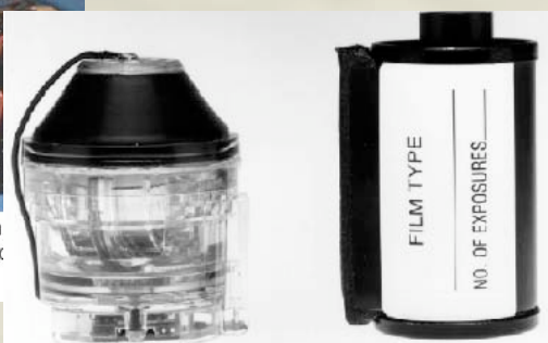
Figure 2.3: The Gyration GyroEngine compares in size favorably with a roll of 35 mm film (courtesy Gyration, Inc.).
