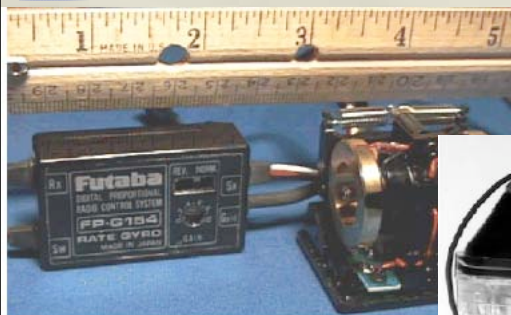
Figure 2.2: The Futaba FP-G154 miniature mechanical gyroscope for radio-controlled helicopters. The unit costs less than $150 and weighs only 102 g (3.6 oz).
