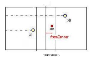
Fig. 12. fromCenter is lower than THRESHOLD, so the robot is on the axis of the docking station.
