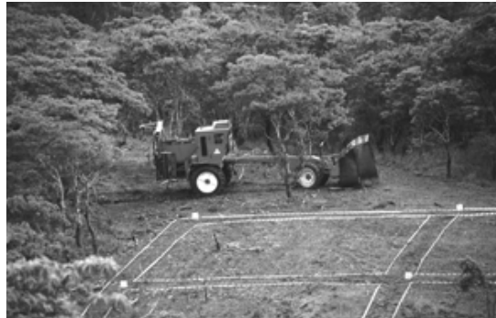
Figure 2 - A minefield being cleared using a large flail
